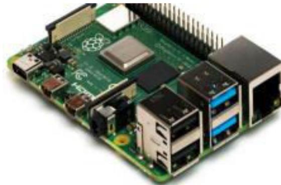
Figure 4.1 Raspberry pi module
